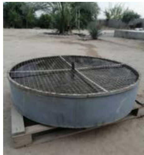
Figure 4 A picture of a type A pan used to measure evaporation in the research
