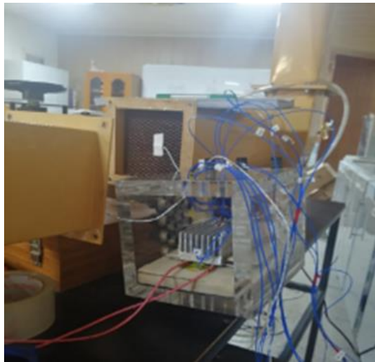
Fig.3 Heat sink inside the test section of the wind tunnel.
