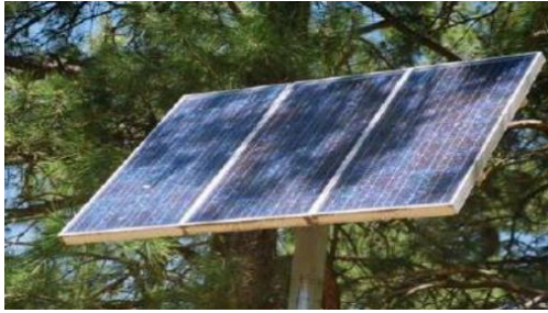
Figure 1. Partial Shading on the PV Panel
