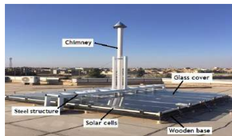
Fig. 4 PV/Solar chimney pilot model
