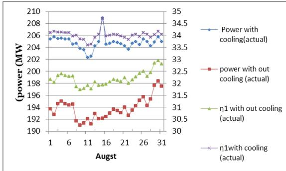
Fig.6-b Gas turbine net power output and  $\eta_1$  with and without cooling system for Augst 2023.(actual data) .
