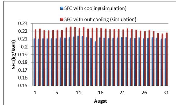
Fig.7-b SFC with and without cooling (simulation data).
