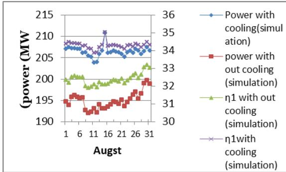
Fig.6-a Gas turbine net power output and  $\eta_1$  with and without cooling system for Augst 2023.(simulation data).
