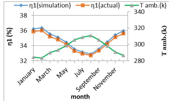
Fig. 4 Thermal efficiency (η<sub>1</sub> ) with ambient temperature for 2023 (actual and simulation data).
