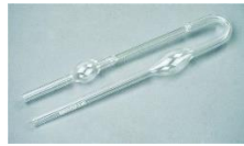
(h) U-tube Viscometer
